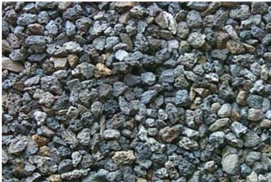
Figure 3.4: Coarse blast furnace slag aggregate (Levy, 2012)
