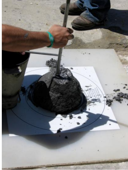
Figure 6.12: Slump of 4” for test mat 3 (Osweiler, 2012)
