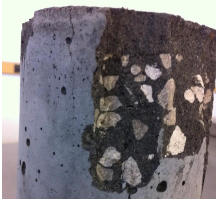
Figure 6.13: Segregation of aggregate and cement paste (Osweiler, 2012)
