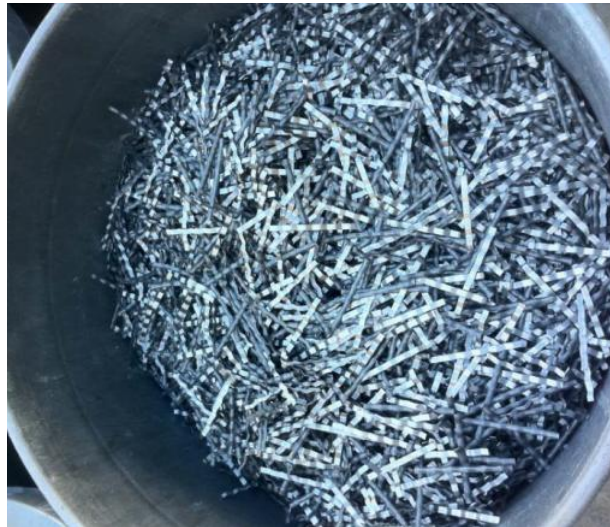
Figure 3.3: Steel fibers used in the conductive concrete test samples (Osweiler, 2012)
