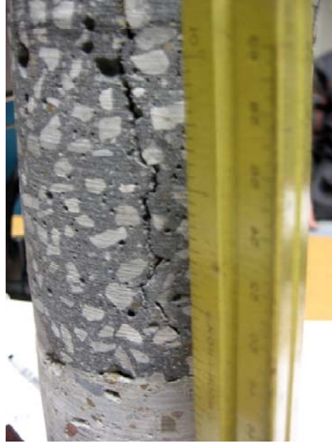
Figure 6.11: Test mat 2 core sample thermal cracking depth (Osweiler, 2012)
