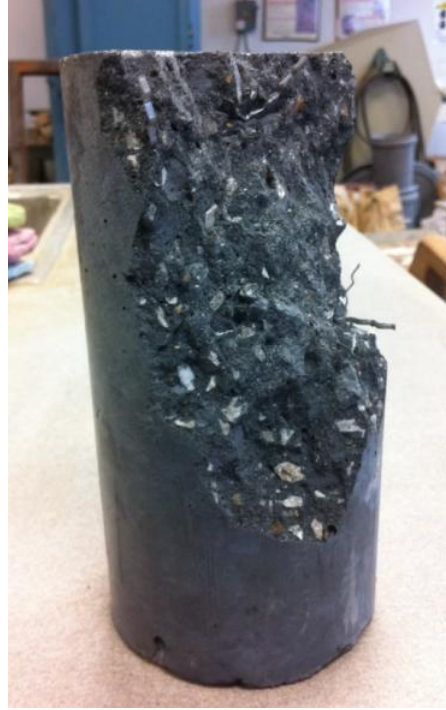
Figure 5.2: Image of materials within conductive concrete mix design (Osweiler, 2012)
